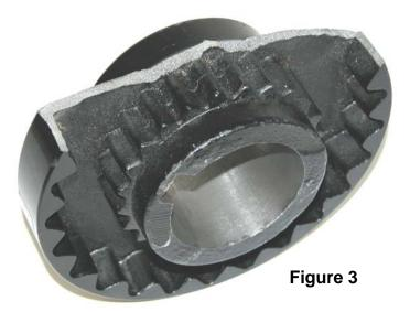
These cracks can fracture during the installation as can be seen in figure 3 or in the presence of any sizable load when placed into operation.
