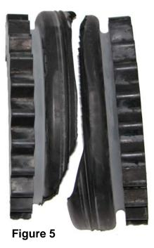
When the elastomeric sleeves is subjected to an excessive load where the torque exceeds the ability of the sleeve to twist, or wind-up, the sleeve will fail or tear in a classical diagonal pattern as shown in figures 4 and 5 as a result of a torque overload. The sleeves are designed to operate with a certain level of wind-up and when the
