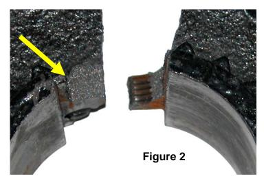
The second condition where this can occur is when a hub is forced onto a shaft in an interference fit condition or the key is too large. The pressure from this interference fit will cause the hub to burst at the weakest point which is typically at one of the top corners of the keyway.
